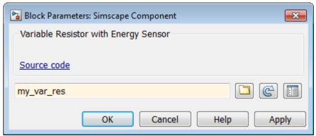
7 Click **OK**. The block icon gets updated, reflecting the selected source component. It now has two conserving electrical ports, + and -, and a physical signal input port PS.
