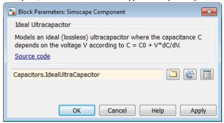
**12** Click **OK**. The block icon in the model diagram updates to reflect the new source component.
