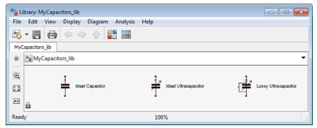
During the library build, if there is an image file in the directory with the same name as the Simscape component file, then this is used to define the icon for the block. For example, the Ideal Capacitor block defined by IdealCapacitor.ssc uses the IdealCapacitor.jpg to define its block icon. If you do not include an image file, then the block displays its name in place of an icon. For details, see "Customize the Block Icon" on page 4-48.
