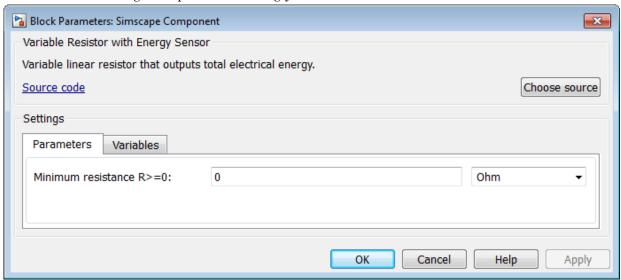
11 Declare the output e and add the equation calculating total electrical energy. The component source now looks like this:
