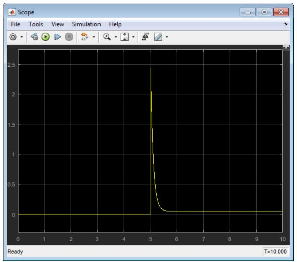
Simulation results show that, when the switch is flipped at t=5 seconds, the current delivered to the load is less than  $2.5~\rm A.$
