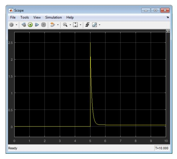
The Simscape Component block points to an ideal capacitor component. Simulation results show that, when the switch is flipped at t=5 seconds, the capacitor delivers 2.5 A to the load.
