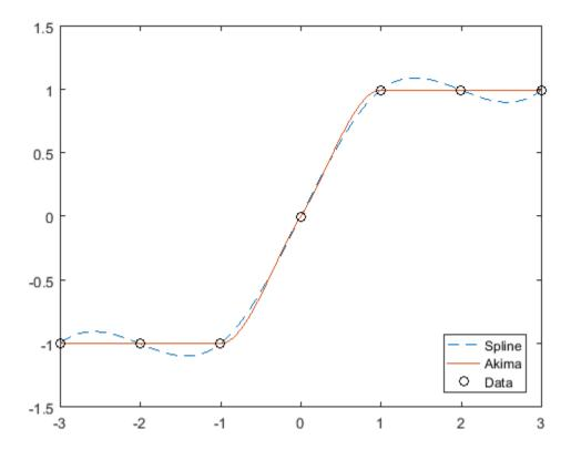
When two flat regions with different slopes meet, it is not possible to avoid an undulation while maintaining smoothness. The original Akima algorithm gives equal weights to the points on both sides, thus evenly dividing the undulation. The modified algorithm, used in this function, gives more weight to the side where the slope is closer to zero. This modification gives priority to the side that is closer to horizontal, which is more intuitive (see next graphic).
